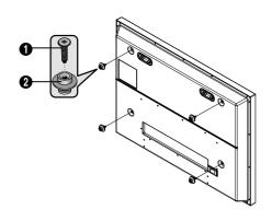
Put the 4 insulation holders on the PDP in the grooves of the wall mount bracket and pull down on the PDP (1) to secure it to the wall mount bracket (2). Tighten the screws as shown (3) so that the PDP cannot be separated from wall mount bracket.
